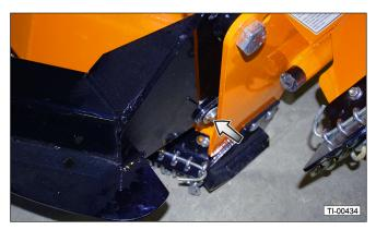
**Note:** If necessary, lengthen the leveling rods by turning the adjustment at the rear of the rods. This will increase the clearance between the leveling rod pin and the hitch pivot bracket.
