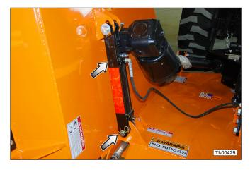
3. Remove the pin, washers, and cotter pins from the front of both leveling rods.
