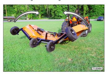
**NOTE:** The center deck will raise fully up before the wing cylinders start to fold the wings.
