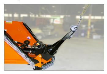
6. Remove the jack from its storage location on the left wing and install it on the lug on the left side of the hitch.
