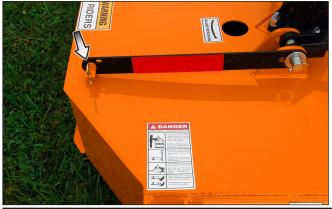
5. Remove the blocking and lower the wings to their operating position.
