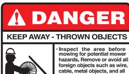
Foreign material can be thrown from the mower and cause serious bodily injury to the operator and passersby.
