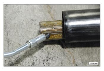
6. Slide the front driveline half over the rear half. Align the square rib on the mating halves to engage.
