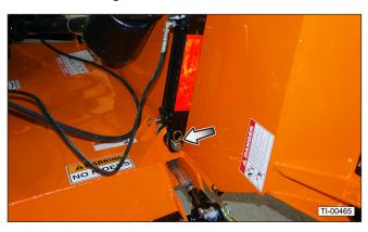
Loosen the lock nuts on the wing stop bolt on one wing, and make sure the wing stop bolt does not touch the wing.
