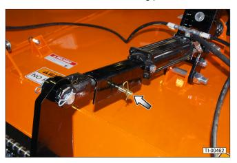
4. Make sure the jack stand is secured in its storage location on the left wing deck.
