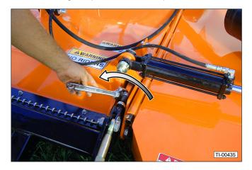
17. Adjust the leveling rods to have equal amounts of tension. This will be a starting point for a later leveling adjustment.
