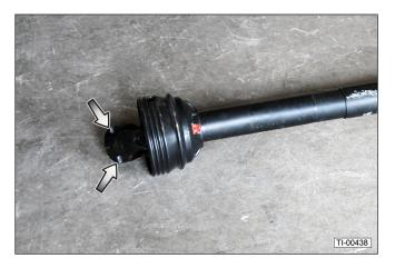
2. Install the driveline onto the gearbox input shaft. Insert the retaining bolts in opposite directions from each other, and tighten the locknuts securely.
